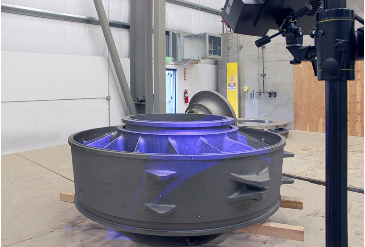
Fig. 3: Blue Light Technology, the narrow-band blue light of the projection unit, allows measurements to be taken independent of ambient lighting conditions and better scanning of shiny surfaces.
